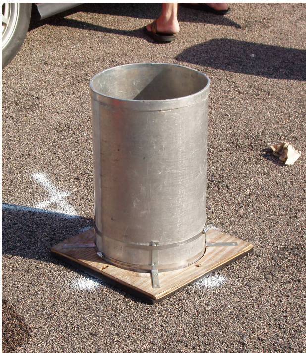
Infiltration tests can be performed to determine the rate at which an area is draining. Image courtesy of URI NEMO.
