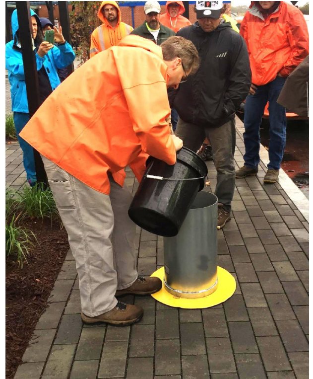
Infiltration tests can be performed on any sort of permeable pavement to determine the rate at which an area is draining. Image courtesy of Coastal Green & Resilient Infrastructure Project.
