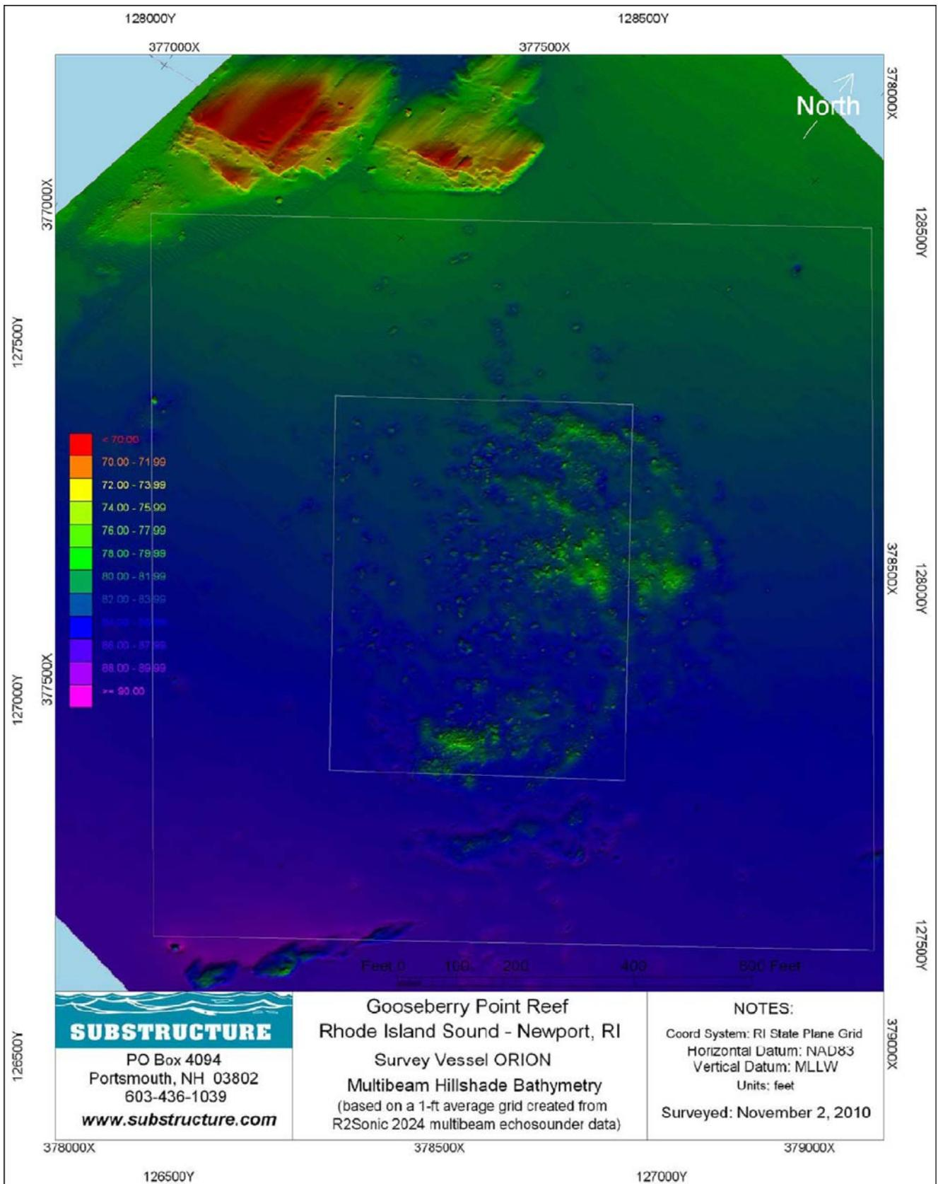
Figure 6. Multibeam Hillshade Bathymetry at Gooseberry Island Reef, November 2, 2010
