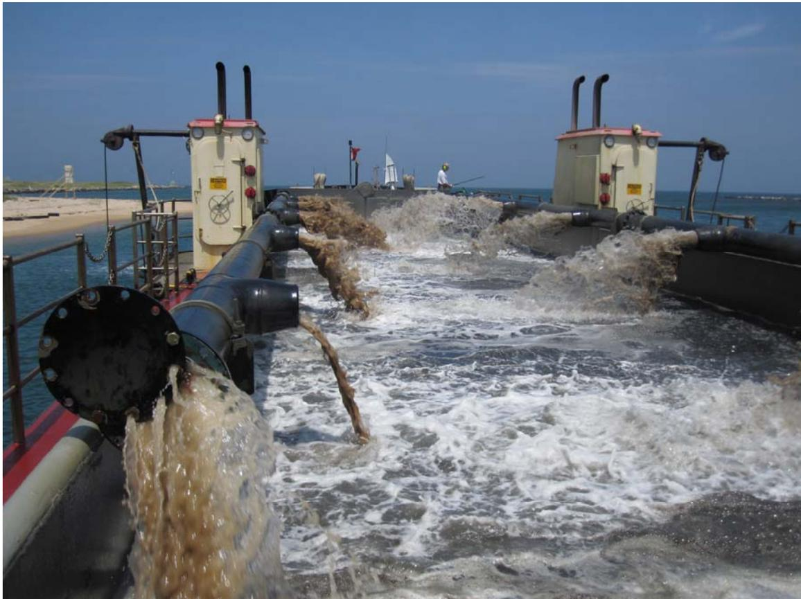
View from the deck of the CURRITUCK during the dredging of the Great Salt Pond Federal Navigation Channel, Block Island (RI) on June 1, 2010 (picture by Eric Schneider, DFW). The CURRITUCK is a special government owned (U.S. Army Corps. of Engineers) small hopper vessel with a split-haul and two hydraulic dredges.
