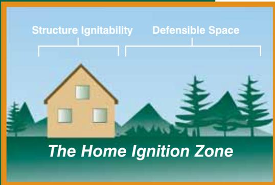
Figure 6: Addressing both components in the Home Ignition Zone will provide the best protection for your home. Credit: CSFS
