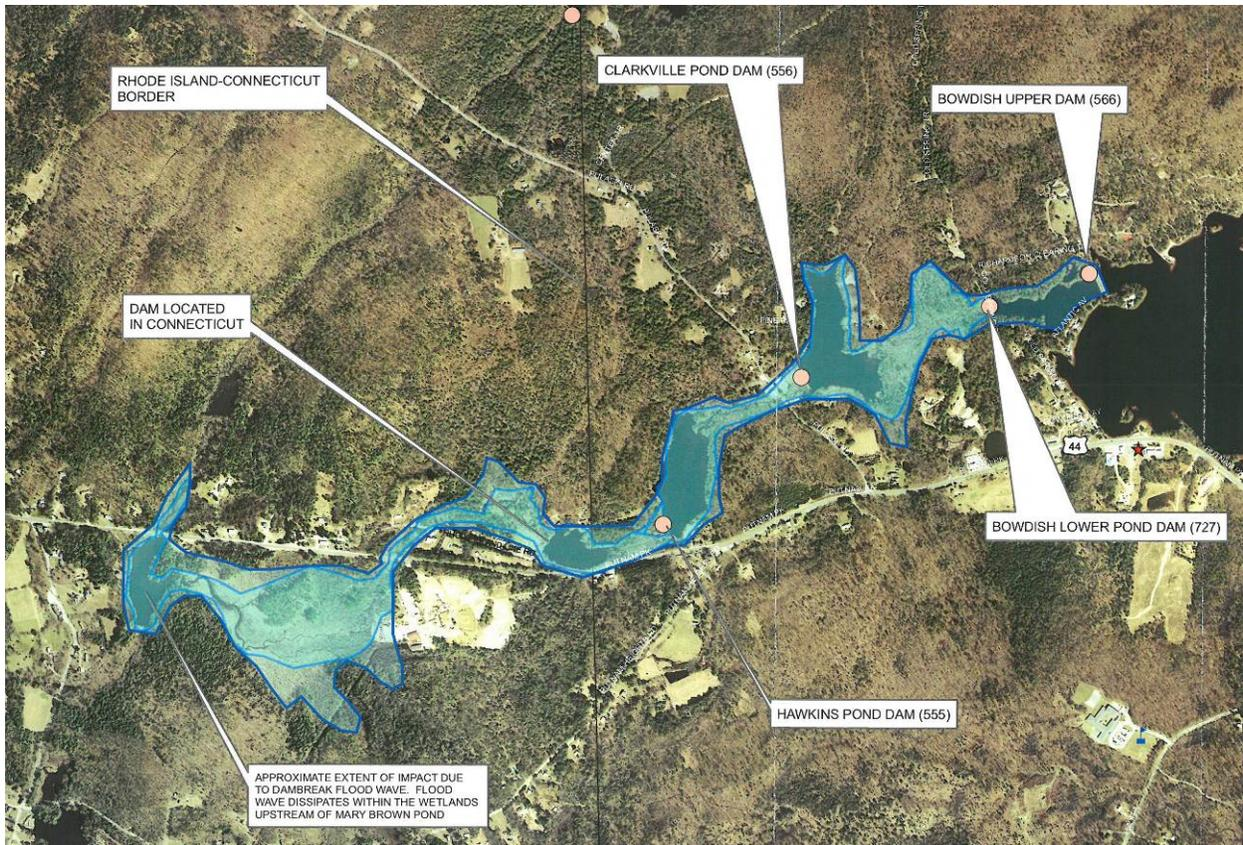
Dam failure inundation map for Bowdish Dam (No. 566), Gloucester. A map specific to each dam is included in the EAP for that dam.
