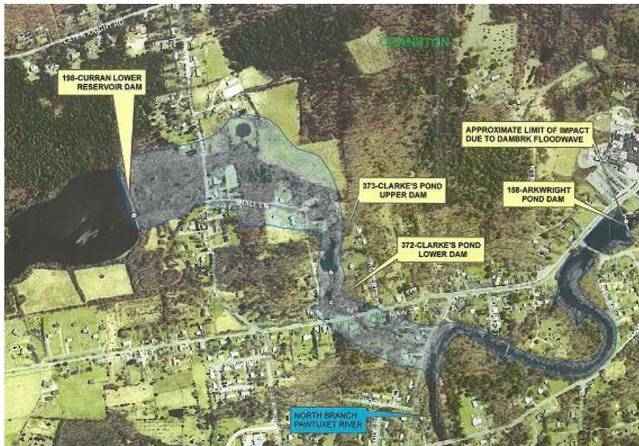
*Hypothetical flood due to catastrophic failure of Curran Lower Dam (No. 198) in Cranston*
