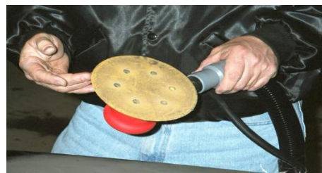
Vacuum holes for sander. Note the vacuum hose attached to sanding unit. Sanding dust is collected in a container nearby, or in a central location.
