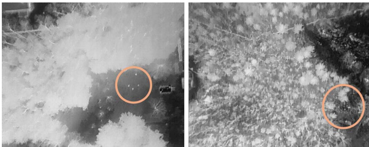
Figure 11. Increased flight altitude negatively affected the ability to confidently detect deer in the imagery. The image on the left was captured at 189m AGL and was estimated to contain 4 deer with high confidence. The image on the right was captured at 350m AGL and also estimated to contain 4 deer, but with low confidence.
