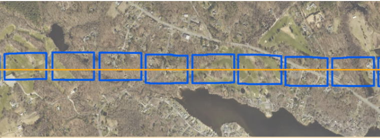
Figure 3. Example of final sequence footprints on the landscape after accounting for overlap between adjacent images and adjacent sequence groups.
