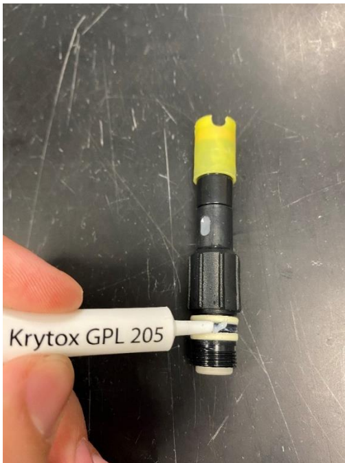
Figure 7 YSI 2030 Probe O-ring with Krytox Grease.
