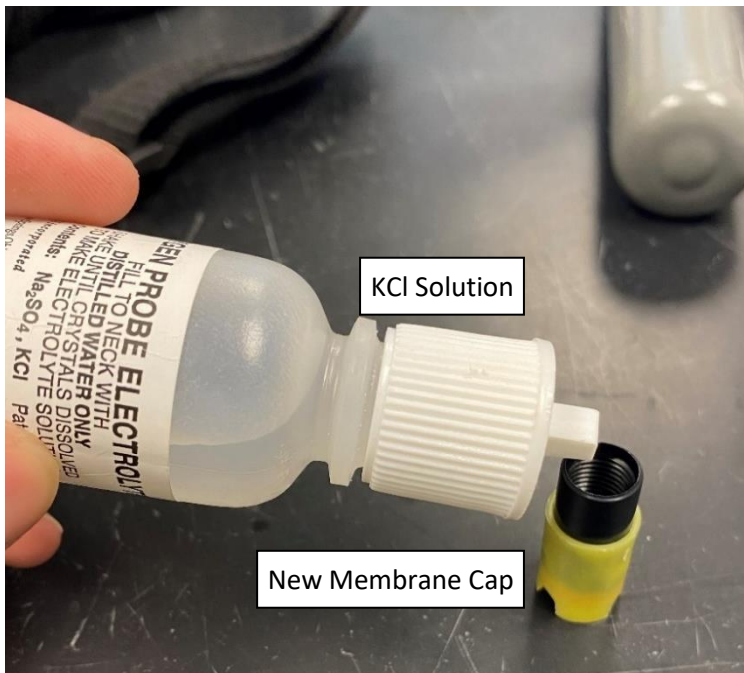
Figure 4 New membrane cap being filled with KCl solution.
