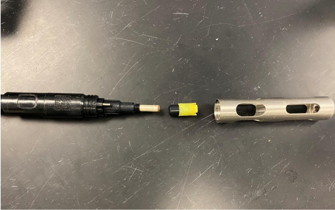
Figure 6 Cleaned and Dried Dissolved Oxygen Sensor Ready for Long-Term Storage.
