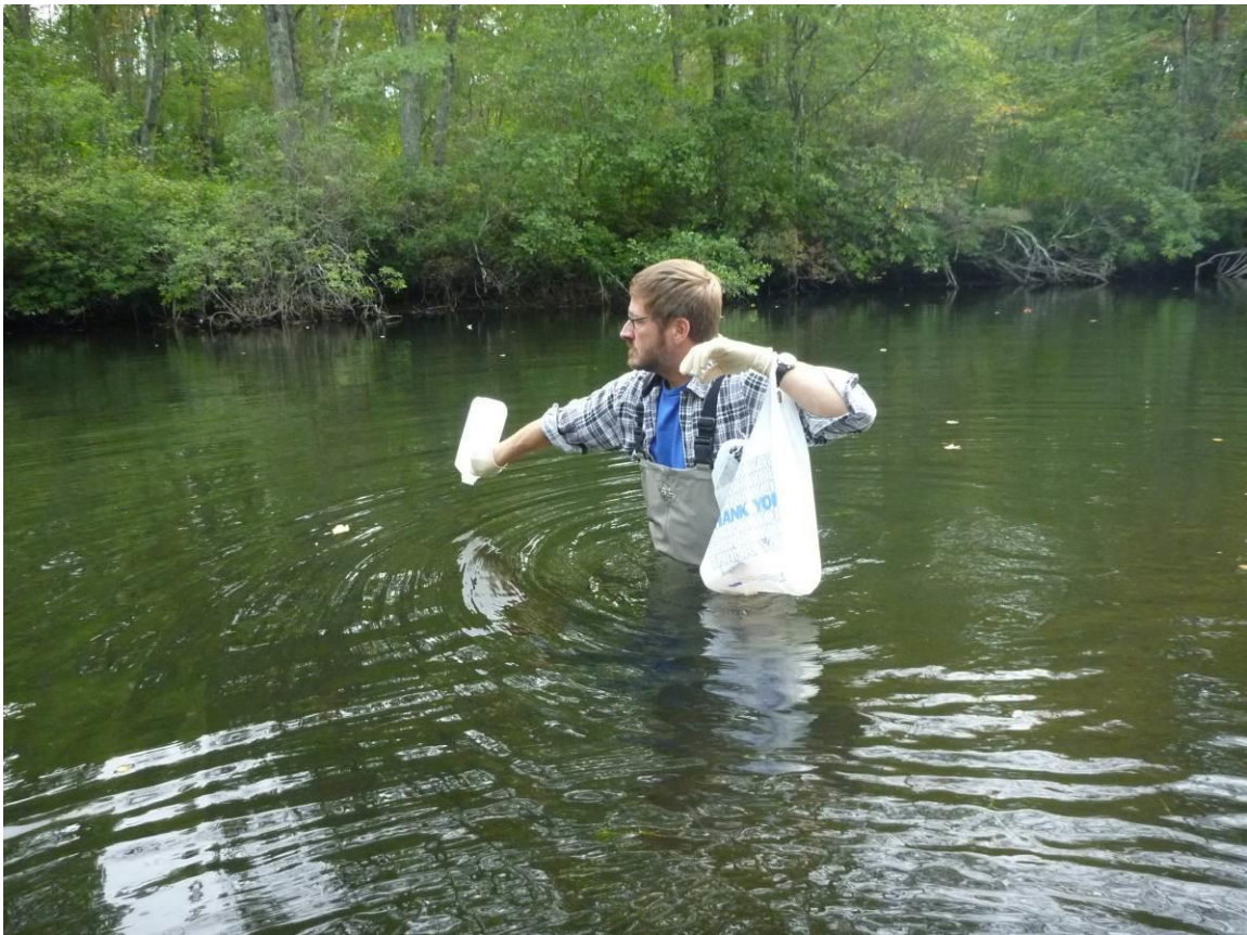
Figure 6 Analyst collecting water using a bottle that is non-preserved, and not a bacteria sample.
