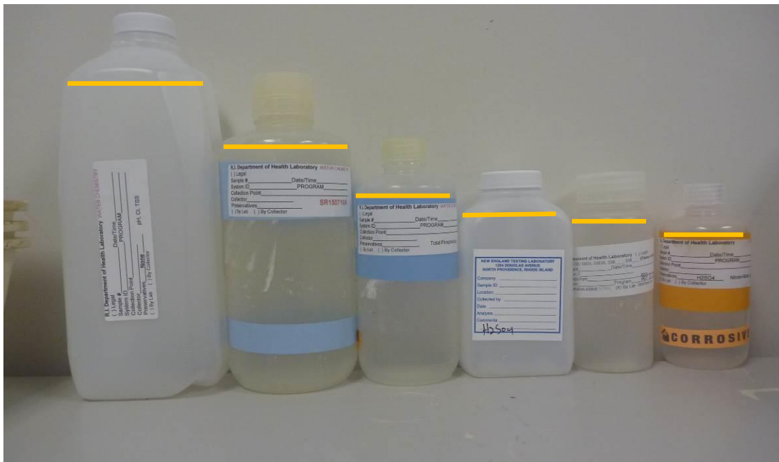
Figure 3 Orange lines are at the shoulder of the various bottles used for the ARM program. Samples should be filled to this level unless program specific instructions are provided.
