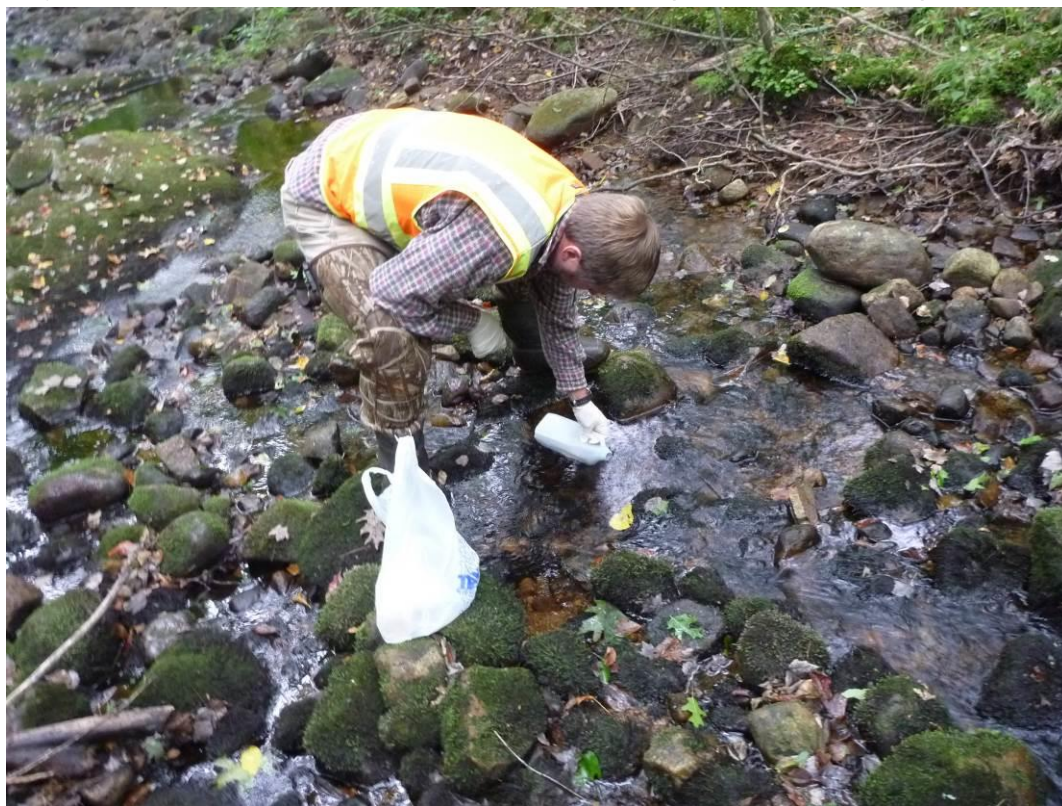
Figure 4 Analyst collecting a sample in shallow water (depth less than 1 foot). This condition should be noted on field sheets.
