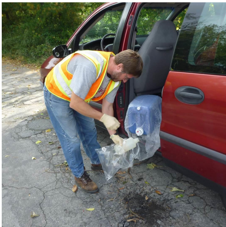
Figure 2. Analyst filling a 1 liter bottle with DIW for a field blank sample.
