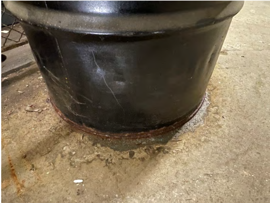
Base of the 55-Gallon Satellite Accumulation Drum (Waste Compressor Oil) – Visible Rust and Staining on the Concrete
