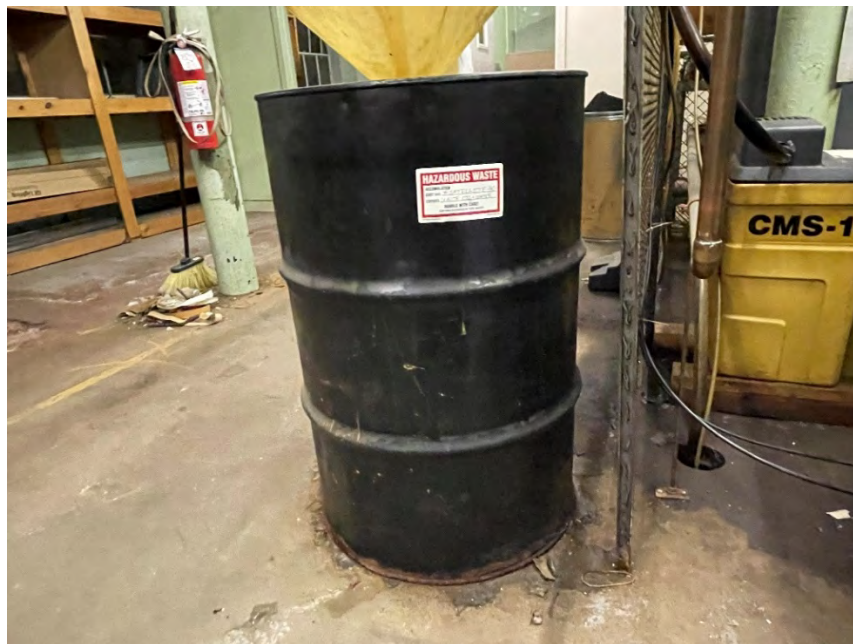
55-Gallon Satellite Accumulation Drum (Waste Compressor Oil) and Staining Around the Floor Drain
