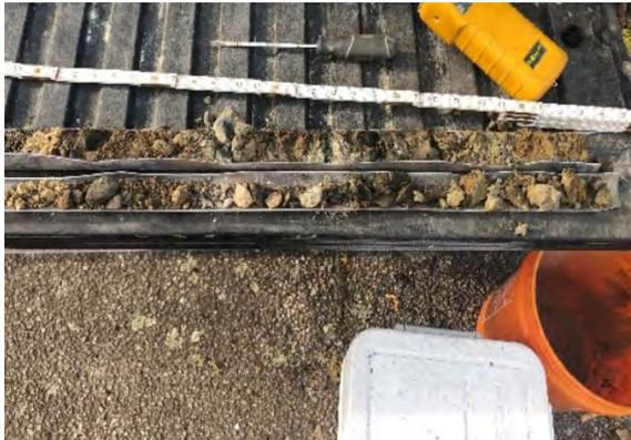
**Photo 15:** SB-11 from 0'-5' bgs. Fill with asphalt, fine to coarse sand, trace silt and cobbles.
