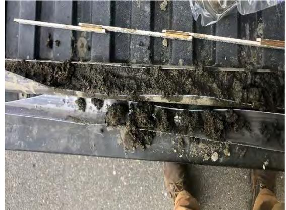
**Photo 2:** SB-2 from 10'-15' bgs. Gray hardpacked sand and trace silt and clay.
