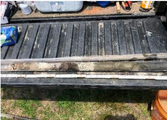
**Photo 9:** SB-8 from 0-5' bgs. Fill with asphalt, sand, crushed stone and trace silt and gravel.
