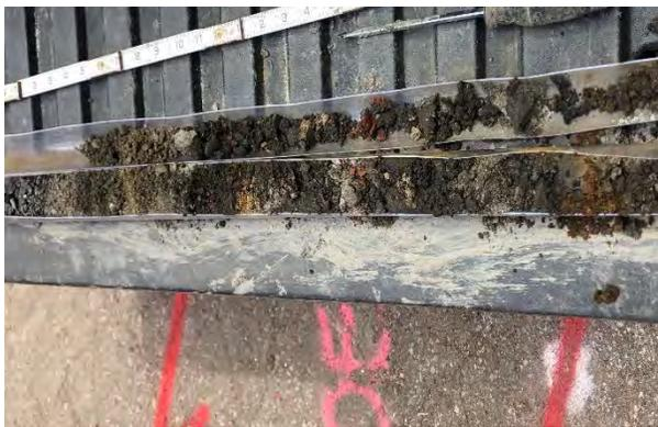
**Photo 5:** SB-4 from 0'-5' bgs. Fill with asphalt, fine to coarse sand and trace crushed stone.
