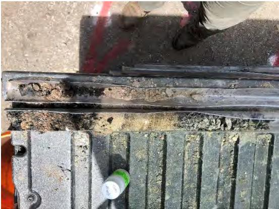
**Photo 7:** SB-5 from 0'-5' bgs. Fill with asphalt, fine to coarse sand and trace silt and ash.
