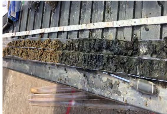
**Photo 6:** SB-4 from 10'-15' bgs. Fine to coarse sand with gray silt and little sand at depth.
