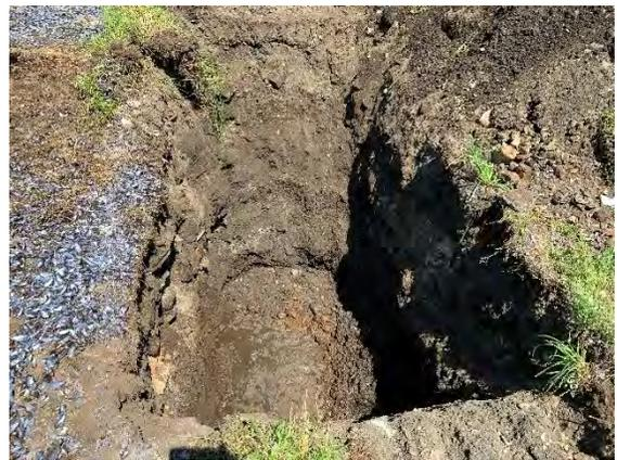
**Photo 18:** TP-3 Fill observed from 0' to 7' bgs.
