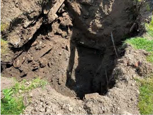
**Photo 19:** TP-6 Fill observed from 0' to 8.5' bgs.
