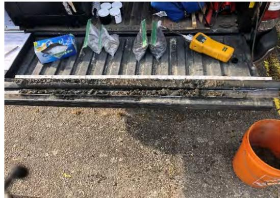
**Photo 16:** SB-11 from 10'-15' bgs. Alternating sand and clayey silt.
