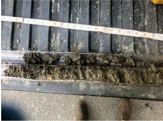
**Photo 1:** SB-2 from 5'-10' bgs. Fine to coarse sand with trace silt.
