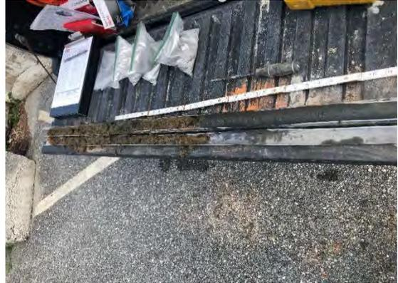
**Photo 14:** SB-10 from 10'-15' bgs. Fine to coarse sand and gray clayey silt with trace gravel
