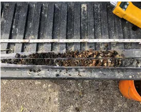
**Photo 11:** SB-9 from 0'-5' bgs. Fill with asphalt, sand with little silt. Trace shells, ash, and glass.
