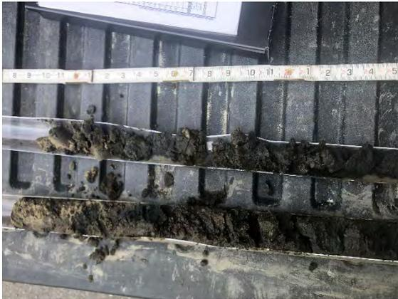
**Photo 3:** SB-3 from 5'-10' bgs. Fine to coarse sand with trace silt and few brick fragments.
