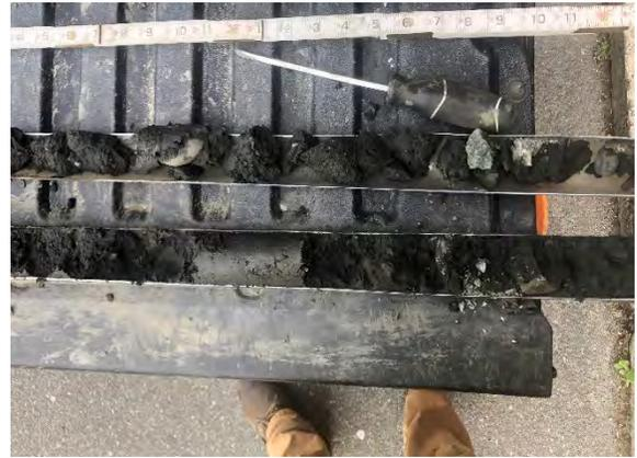
**Photo 4:** SB-3 from 10'-15' bgs. Gray fine to coarse sand and hardpacked silt at depth.
