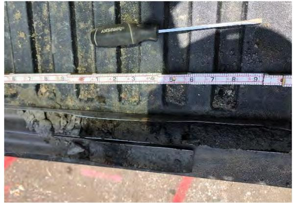
**Photo 8:** SB-5 from 5'-10'. Fine to coarse sand and trace silt. Gravel at 5' depth.
