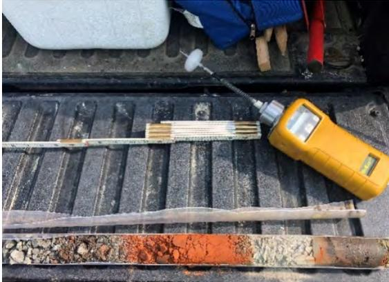
**Photo 13:** SB-10 from 0'-5' bgs. Fill with crushed brick and stone, fine sand, and little silt.
