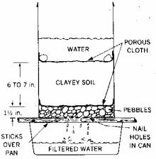
Settling, filtering, and a combination of the two are the easiest and most efficient methods for decontaminating water. These methods should provide sufficient temporary water supplies for the animal handling facility. It is recommended that clean, stored water be used primarily for human consumption and decontaminated water be used for animal consumption. If decontaminated water must be used for human consumption, it should first be disinfected by boiling or by chlorination.
