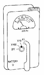
Note the "battery check" button on the face of the survey meter. Pushing this button tells you whether the batteries are good or not. If the button is pushed, the needle should fall within the "BATT CHECK" bar on the survey meter dial. If the needle falls to the left of the "BATT CHECK" bar, the batteries should be replaced before the survey meter is used. Otherwise, the meter will not operate properly.
