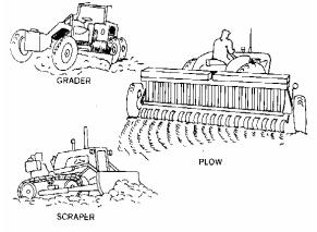
Since it is not feasible to operate large earthmoving equipment in confined areas or around buildings, small garden tractors, or front end loaders equipped with a small scraper can be used for scraping or plowing. Hand labor with shovels and wheelbarrows may be necessary to remove radioactive material from some smaller areas.
