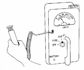
Do not attempt to make radiation measurements unless the survey meter is operating properly. This is one of the most important rules in radiation protection. Since the most common cause of survey meter failure is weak batteries, the condition of the batteries should be checked before each use. After the survey has been completed, and if the survey meter will not be needed for some time, switch it off. This will prolong the life of the batteries.
