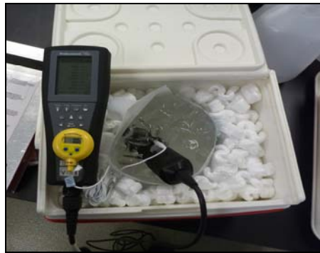
Figure 19. YSI Pro Plus meter in ice/water bath with NIST traceable thermometer.
