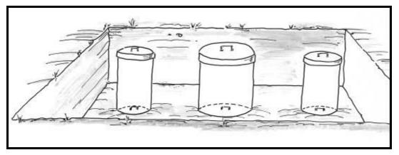
**Figure 4.3b** Proper installation of concrete well ring risers on the main access (manhole). Main access (manhole) cover remains on the tank; well rings are capped with a concrete cover that overlaps the outside of the rings to prevent leakage.
