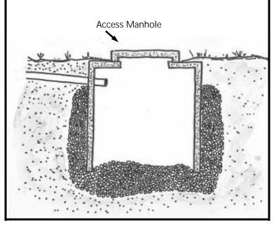
Figure 5.3 Diagram of a cesspool
