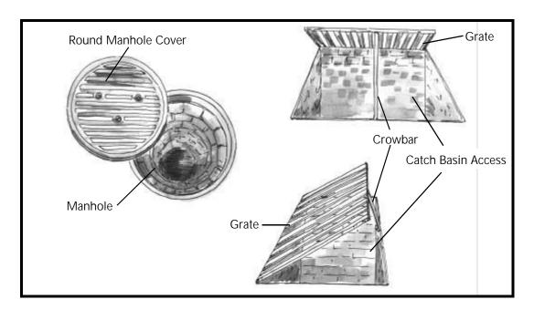
Figure 5.5 Opened storm drain grates.
