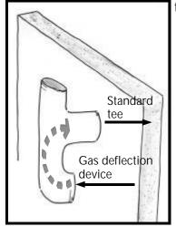
**Figure 4.4** A gas baffle typically employs a standard sanitary tee fitted with a gas deflection device.
