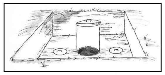
**Figure 4.3c** Improper installation of well ring risers with the septic tank main access (manhole) cover moved to the top of the well ring. This provides a poor fit, which may result in leakage as well as chipping of the concrete.
