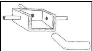
Figure 1.3a Cut-away view of a conventional 1000-gallon septic tank. Wastewater flows by gravity from the building sewer to the septic tank, followed by the distribution box and then to the soil absorption system.
