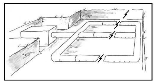
Figure 1.2a Soil absorption bed system
