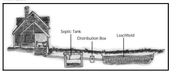
Figure 5.1 Diagram of a conventional septic system
