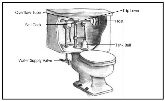
Figure 3.2 Diagram of a toilet
