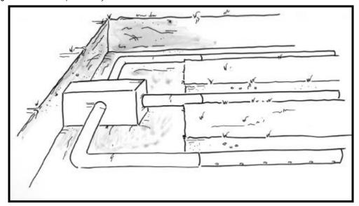
Figure 1.2b Soil absorption trench system
