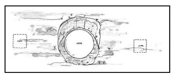
**Figure 4.2b** Top view of a typical unearthed septic tank main access (manhole). (Current regulations require a manhole and two inspection ports. DEM is revising the regulations to require two 20-inch manholes at the influent and effluent ends of the tank and no center manhole.)
