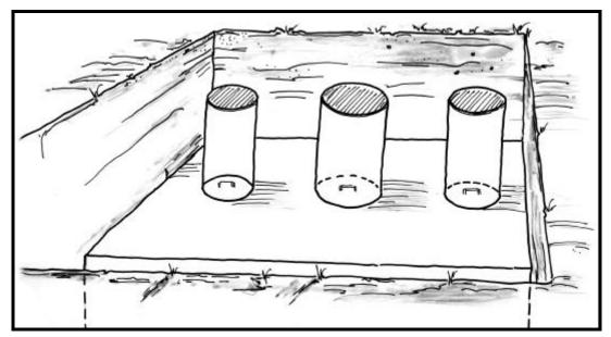
Figure 4.3a Proper installation of fiberglass risers.
