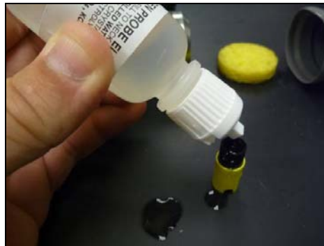
Figure 5. New membrane cap being filled with KCl solution.
