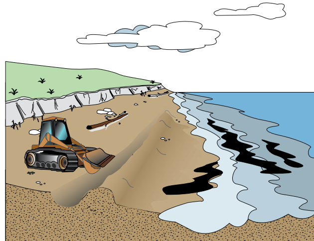
Figure BB-1. Beach berm construction.
