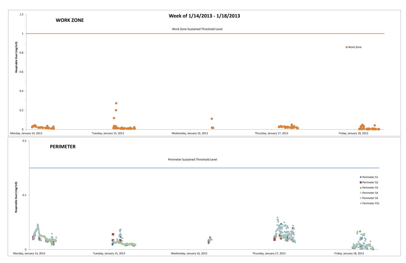
Transient readings were conducted over a three minute time period. A reading is sustained if it is held for over a five minute time period.
