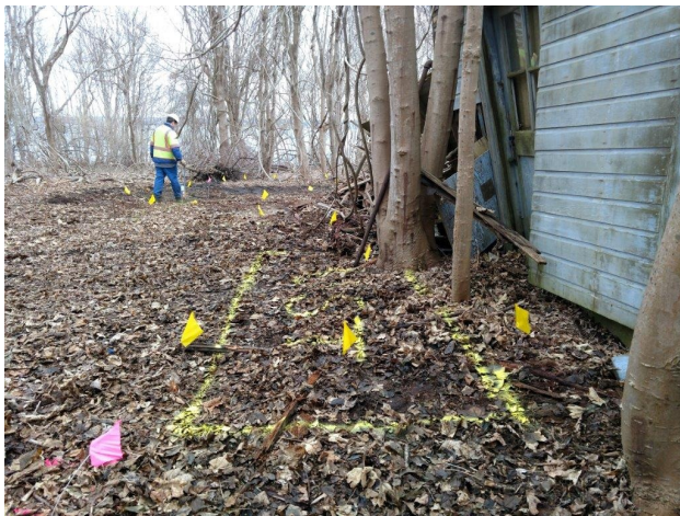
Photograph 3. Northeast of Building 12, view to the east. Building 12 is on the right of the photograph. The probable UST detected in the area of interest is marked with yellow pin flags in the foreground. An area of buried metal is marked with yellow flags in the background, surrounding the operator.
