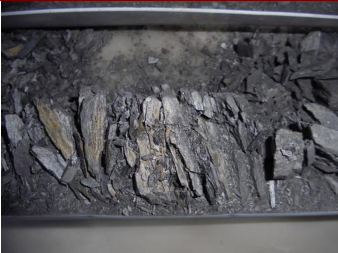
107. Typical image of weathered bedrock overburden at the Site.
