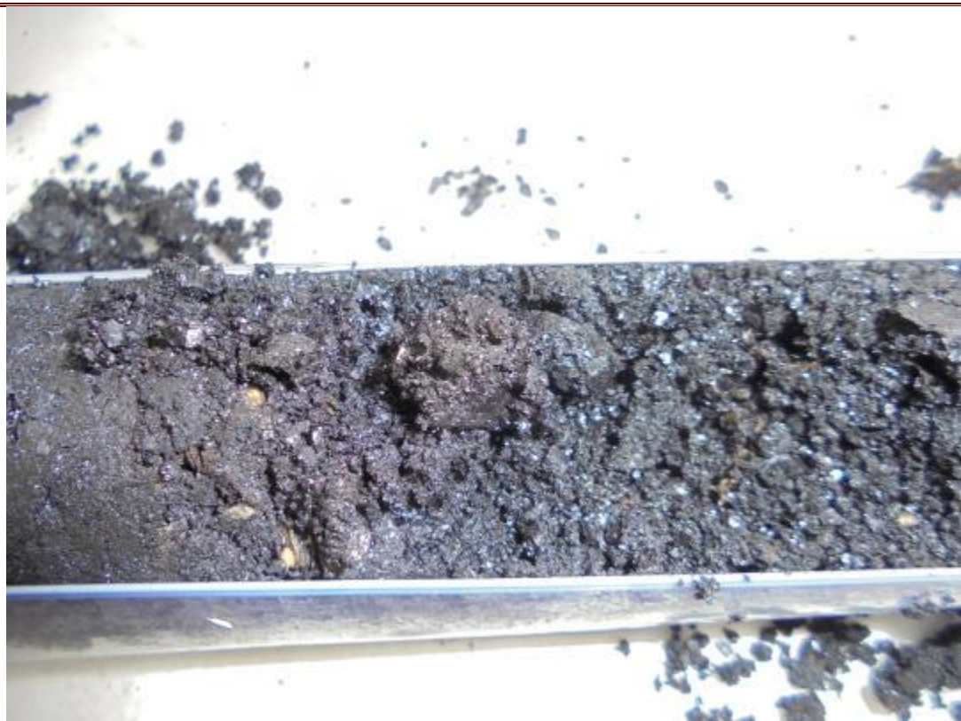
114. Coal comingled with soil in NED Site 23.
