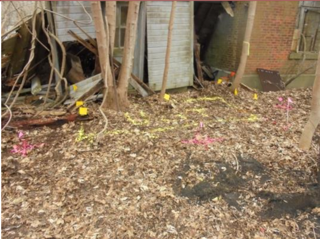
92. Outline of the UST near the northeast corner of NED Site 12 as marked by Hager-Richter during the geophysical survey.
