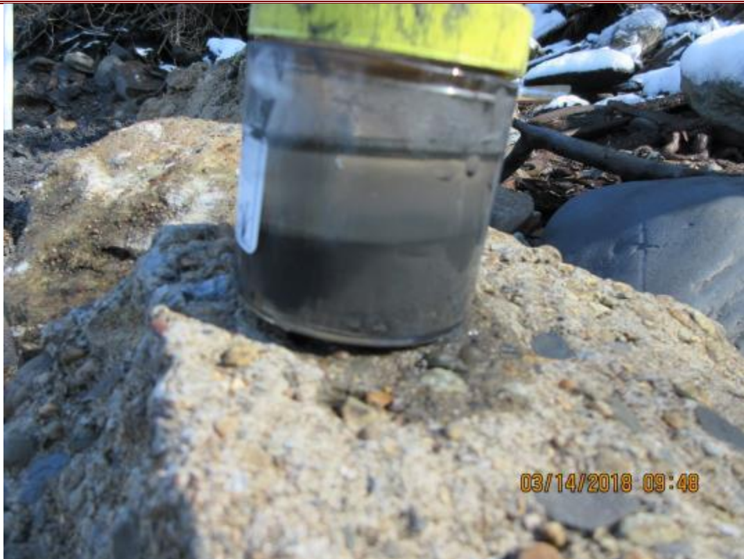
132. Shake test for free product in 10TP8 peizometer location. No free product observed, slight sheen.
