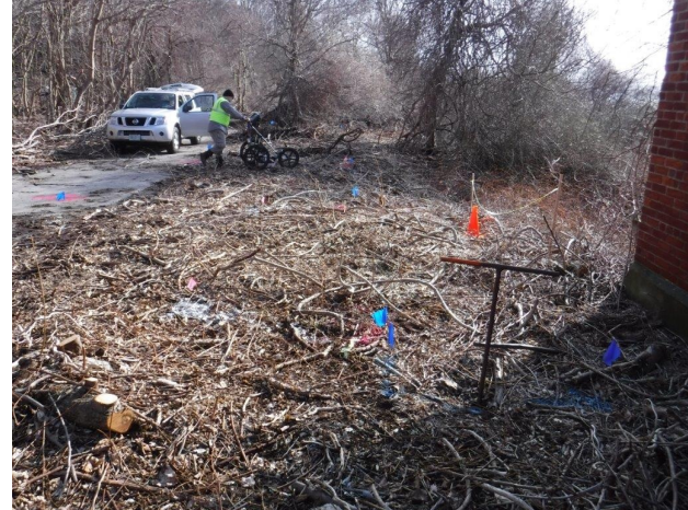
Photograph 2. Area adjacent to Building 8 (visible on right side of photograph), view to the south. The area in the foreground and center of the photograph have been cleared of brush. The operator is pushing the GPR cart.
