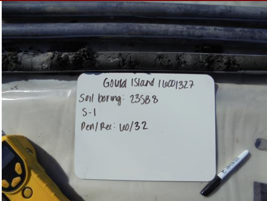
105. A typical soil macrocore collected from the Site.
