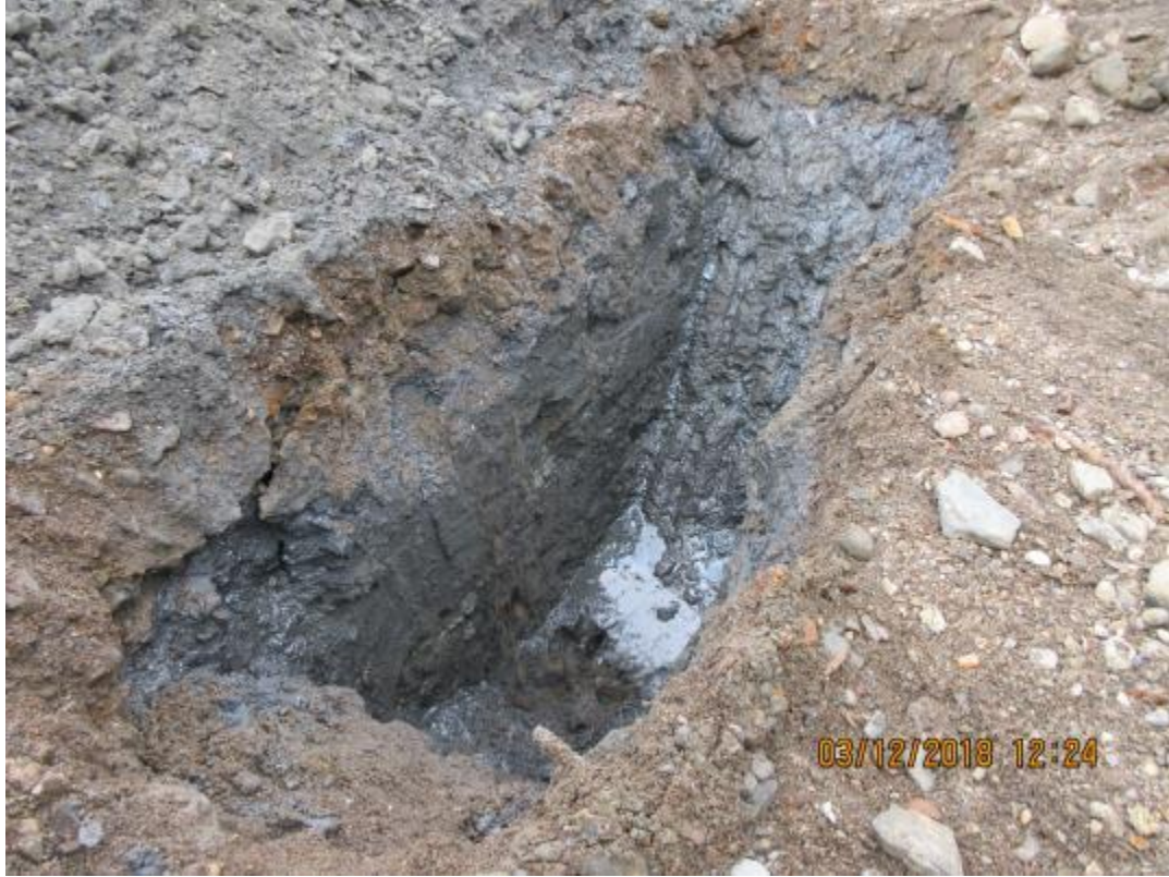
129. 10TP8 with sheen percolating into excavation from 1 foot bgs.
