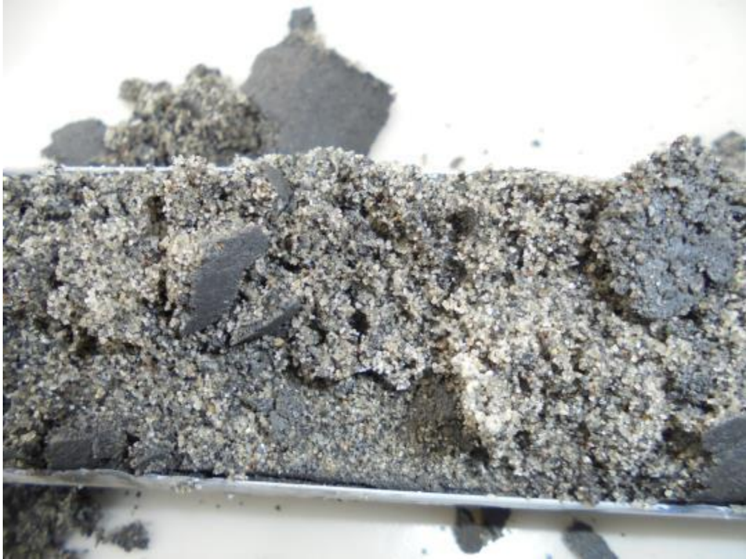
109. Typical gray sandy soil encountered beneath the aviation pad.
