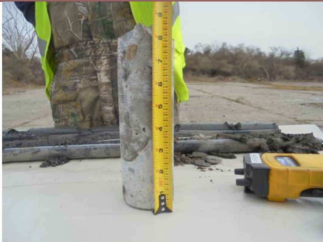
106. Typical concrete core from the aviation pad.
