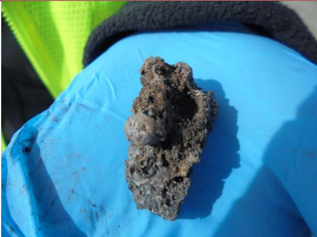
108. Clinker observed beneath the aviation pad.
