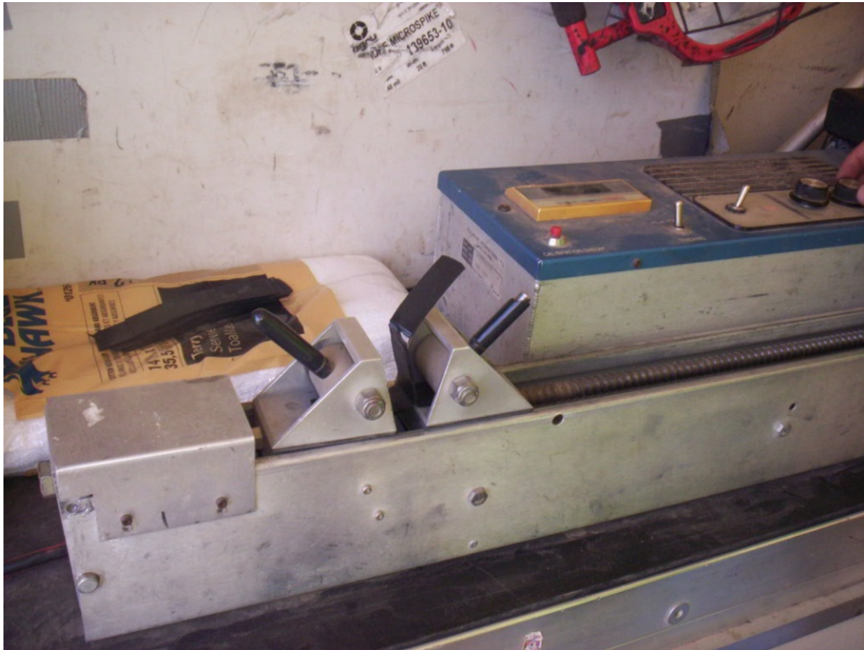
Date Photo ID Description 10/23/12 1590 On-site testing equipment for peel and shear tests
