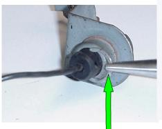
4. Remove the clip that secures the mercury switch holder by pulling the clip off with a pair of needle nose pliers
