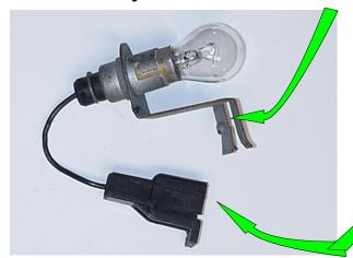
2. Remove the power source by pulling the lighting assembly connector out of its mating connector by hand
