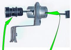
5. Remove the mercury switch holder by pushing it out of the assembly from the wired end
