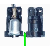
7. Pry the plastic switch holder apart along the center line using a screwdriver and replace the mercury switch with a ball-bearing switch oriented with the rounded end toward the wire contact of the plastic holder.
