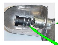
2. Remove the clip that secures the mercury switch holder in the lighting assembly by pulling the clip off with a pair of needle nose pliers
