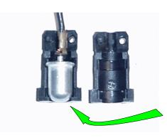
5. Pry the plastic switch holder apart along the center line using a screwdriver and replace the mercury switch with a ball-bearing switch, oriented with the rounded end toward the flanged end of the plastic holder.
