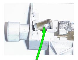
5. Push the mercury switch holder back into place with a screwdriver and adjust the position of the switch to have the center conductor touch the copper strip on the assembly wall
