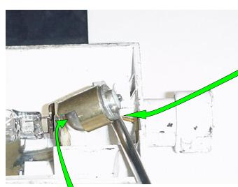
4. Push the mercury switch out of the holder using a screwdriver and replace the mercury switch with a ball-bearing switch oriented as shown 3. Pry up the mercury switch holder with a small screwdriver
