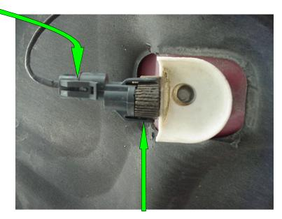
2. Remove the mercury switch holder from the back of the lighting assembly by sliding a screwdriver under the two wing clips and pulling until the switch holder clears the copper rod on the attached section
