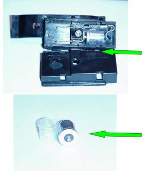
2. Remove the power source by lifting the wiring connector over the tab and pulling the wirng harness off the lighting assembly.
