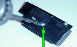
4. Use a drill with a 3/8" bit to remove the head of the pop-rivet that secures the two halves of the assembly.
