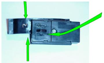
3. Remove the bulb from the assembly by pulling it from socket
