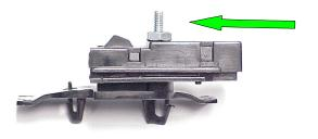
7. Remove the old pop rivet. Snap the casing back together. Then use a 1" #8-32 bolt and #8-32 nut to replace the pop-rivet and tighten to secure the assembly. Snap the assembly back into place, reattach wiring clip, and insert bulb. Verify that the switch is actuating properly.
