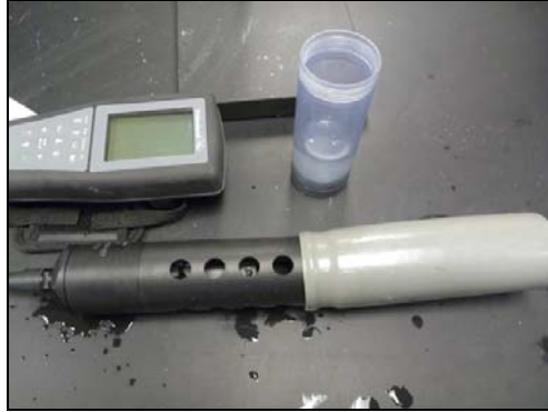
Figure 21. YSI Pro Plus with sensor guard and storage sleeve.
