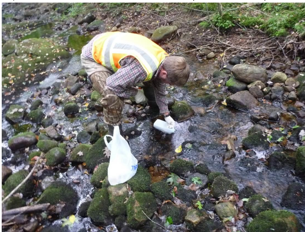
Figure 4 Analyst collecting a sample in shallow water (depth less than 1 foot). This condition should be noted on field sheets.
