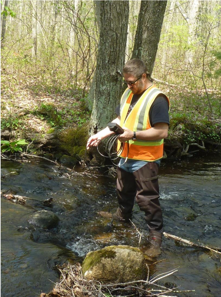
Figure 6 Using YSI Multi-Parameter Meter in Stream.
