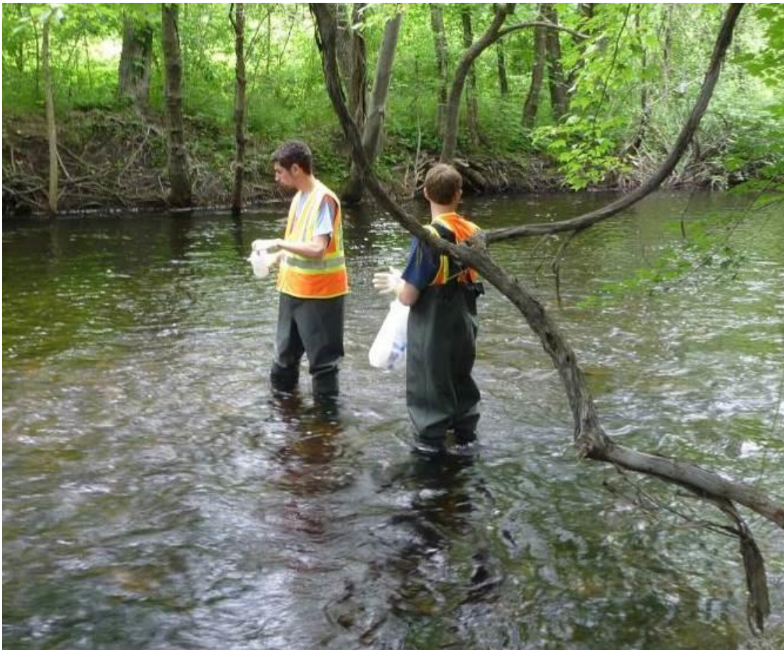
Figure 5 Clean hands person on the left of picture only handles bottles with clean gloves after entering water.
