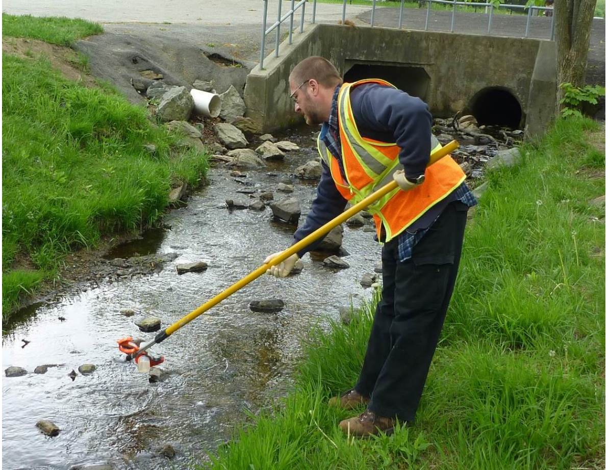
Figure 8 Analyst collecting a water sample from the streambank using the sampling wand.
