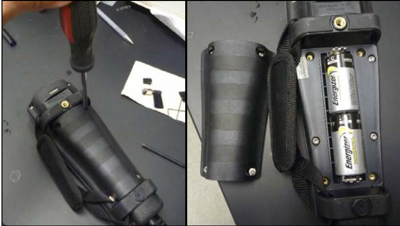
Figure 3. The battery compartment of the YSI Pro Plus, accessed using Philips head screwdriver.
