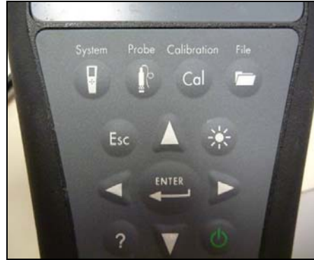
Figure 7. YSI Pro Plus instrument panel.
