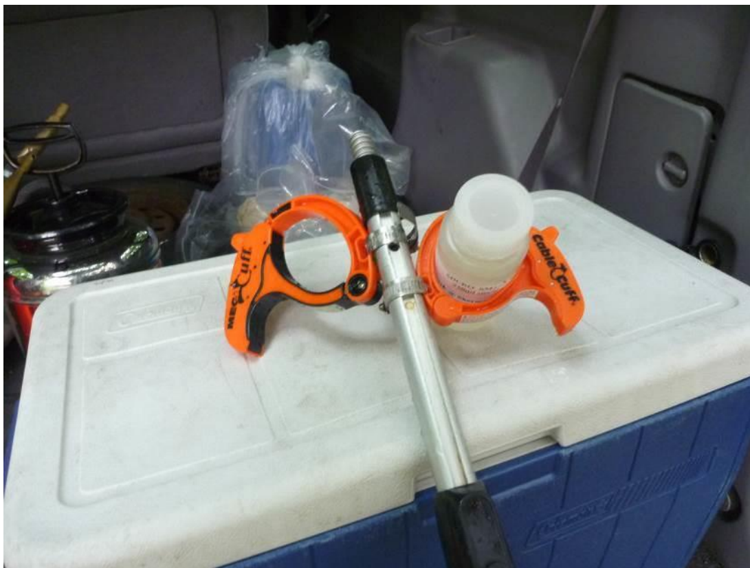
Figure 7 Sampling wand with bottle inserted in small clip.
