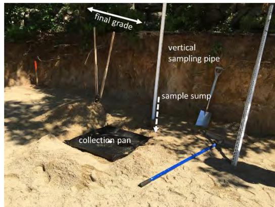
Pan lysimeters will be fabricated and installed by staff of Barnstable County Department of Health and Environment. The vertical sampling port will be protected by a standard curb box. Other sampling ports may be required.
