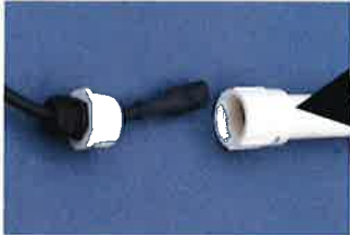
Top End of PVC Handle with newly bonded adapter
