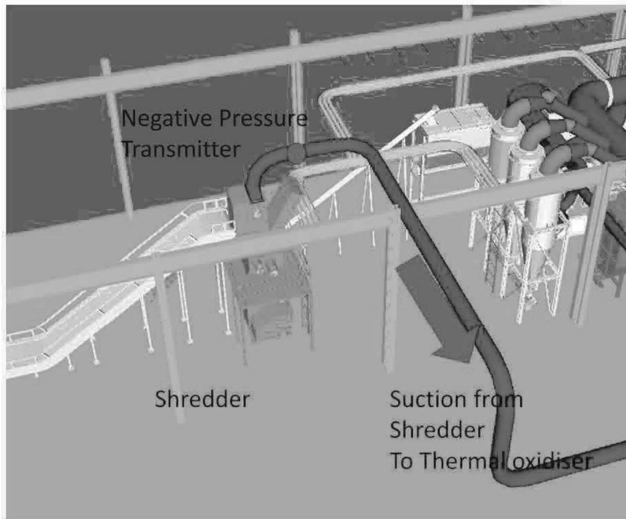
Note all areas prior to thermal degradation are sealed and
