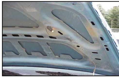
Placement of light switch in hood
