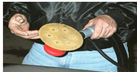
Vacuum holes for sander. Note the vacuum hose attached to sanding unit. Sanding dust is collected in a container nearby, or in a central location.
