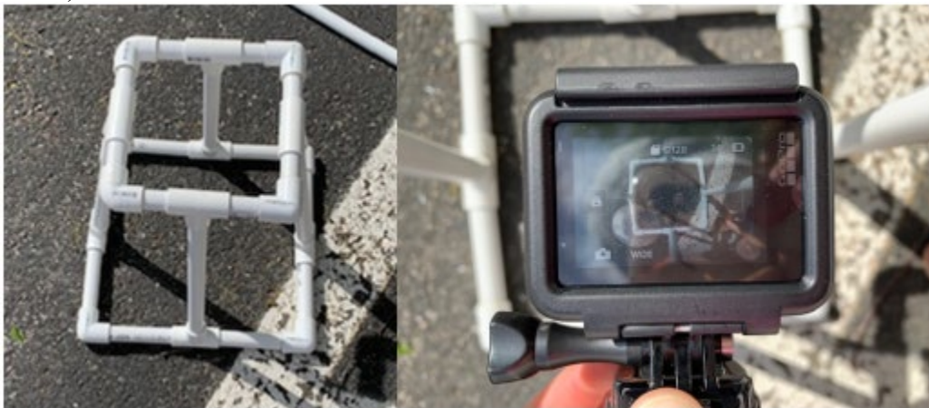
Figure 1. Image of photoquadrat set up and GoPro view.
