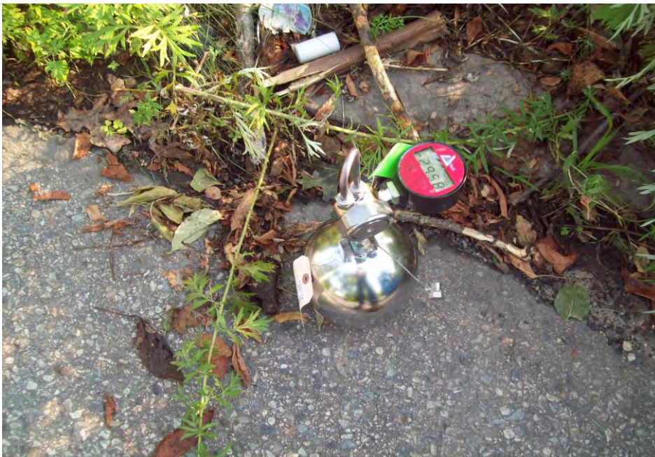
Typical SUMMA canister placement.
