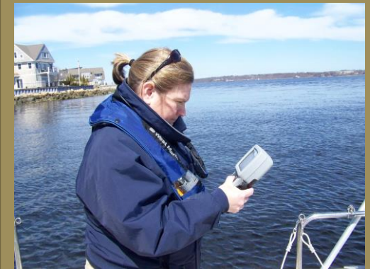
A scientist from NBC taking dissolved oxygen measurements using a YSI sonde. Photo courtesy of NBC.
