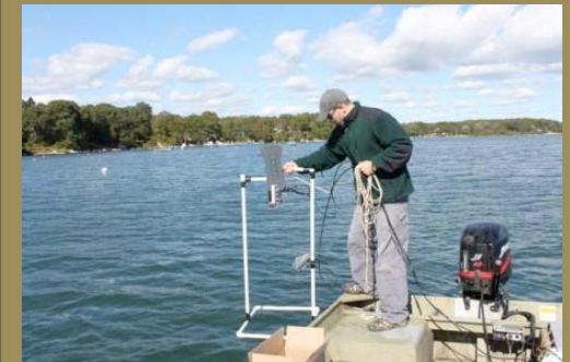
The underwater video camera and quadrat-frame used to map eelgrass as part of the Tier-2 Rapid Assessment. Photo courtesy of NBNERR.
